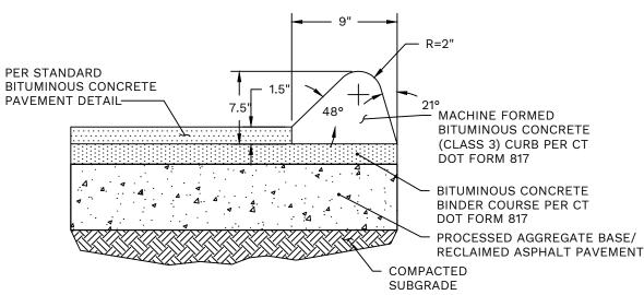
BITUMINOUS CONCRETE LIP CURB NOT TO SCALE
